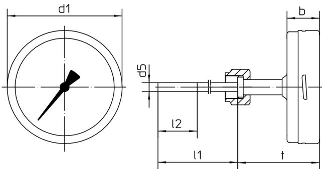
The sensitive portion l2 shall reach the media temperature completely.
