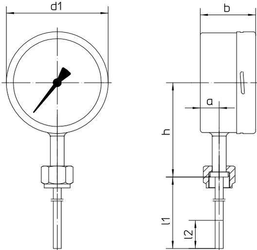
The sensitive portion l2 shall reach the media temperature completely.
