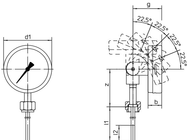
The sensitive portion l2 shall reach the media temperature completely.
